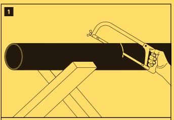
Use a hacksaw to cut the metal pipe into lengths of about 4 ft. shorter ones are possible, but make access to the 'cuffs' easier.
