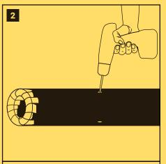
File down and pad the ends with foam and gaffer tape, and drill holes in both sides.
