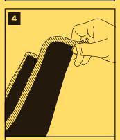
Use a single length of foam insulation to fold over the edges of the bottle until it is completely covered.
