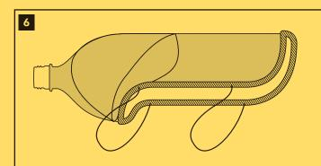
Make four small holes in the sides of the mask. Feed the ends of the elastic bands through the holes and tie them off so they can be pulled back through. Seal the holes with glue to prevent leaks in the mask. Carry a bottle of vinegar to soak the mouth cover before putting on the mask.
