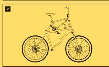
Sit one bike on top of the other and weld them together. Add extra material to strengthen, and join the forks together so the top bike steers the bottom. Add a new chain and brakes so the top bike drives the bottom one. Repeat with two more bikes. The pair of top bikes and the pair of bottom bikes should match as closely as possible.
