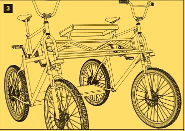
Weld in a connecting frame for people to stand on, and another near the front of the bike to make the entire unit into a rigid structure.
